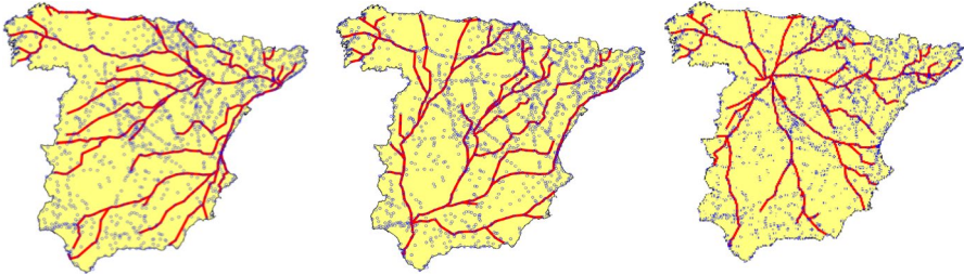
Fig. 18 Optimal networks depend on the city they refer to. Calculation of the optimal networks for three cities: Barcelona, Seville and Valladolid using the procedure described in the text, based on the Dijkstra (1959) algorithm
