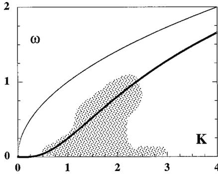
FIG. 1. Schematic phase diagram in the  $\omega$  vs  $K$  plane showing (dotted area) values of the parameters for which a mode-locking motion of the kink at some value of the intensity of the external force  $F_{ac}$  is found (here  $\alpha=0.1$ ). Upper and lower curves show the phonon band gap and the Peierls-Nabarro frequency, respectively.
